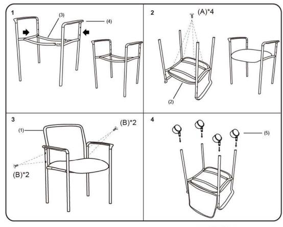
PLEASE NOTE: Do not fully tighten all screws until chair is fully assembled.
